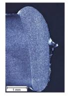
Emitter distance: 3 mm Heating time: 20 s Melt layer thickness: ~ 1,1 mm = const. (transmitted light microscopically photo with polarized light)
